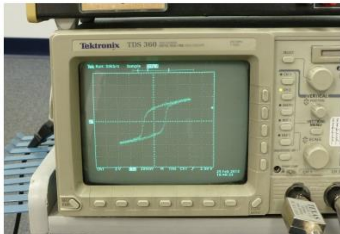
Figure 5: A real-time hysteresis loop displayed on a digital oscilloscope [7], [12].
